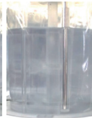
Figure 7: Determining the mixing time based on the decolourisation method using a video camera.
