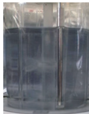
Figure 7: Determining the mixing time based on the decolourisation method using a video camera.
