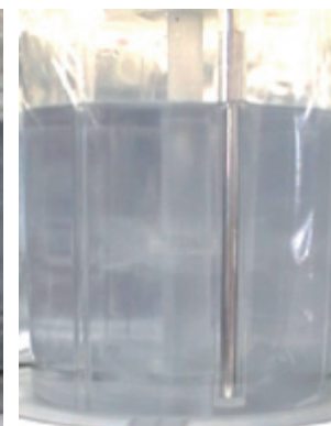
Figure 7: Determining the mixing time based on the decolourisation method using a video camera.
